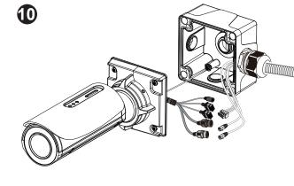
Secure the camera to box using the T25 torx wrench.
